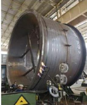
Bearing Housings – Fabrication in progress
