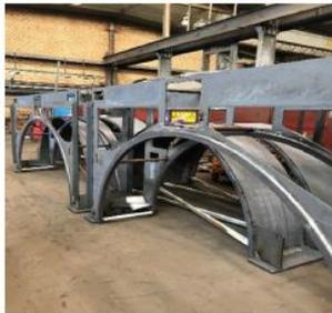
Ball Mill Shell Feed Section – NDT of Circumferential Welds in progress
