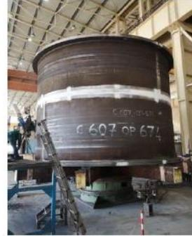
Ball Mill Shell Discharge Section – Circumferential Welding in progress
