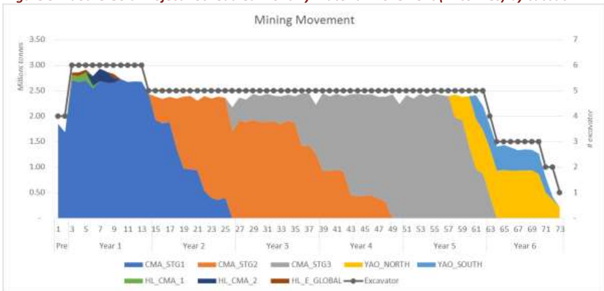
Figure 5: Yaouré Gold Project - Scheduled monthly material movement (M tonnes) by cutback
