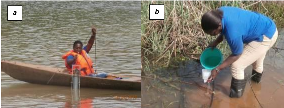
Figure 2-4: Sampling sessions: (a) using the hydrologic bottle, and (b) using the filtration bottle (Photo: KONAN K. Félix; April 2015)
