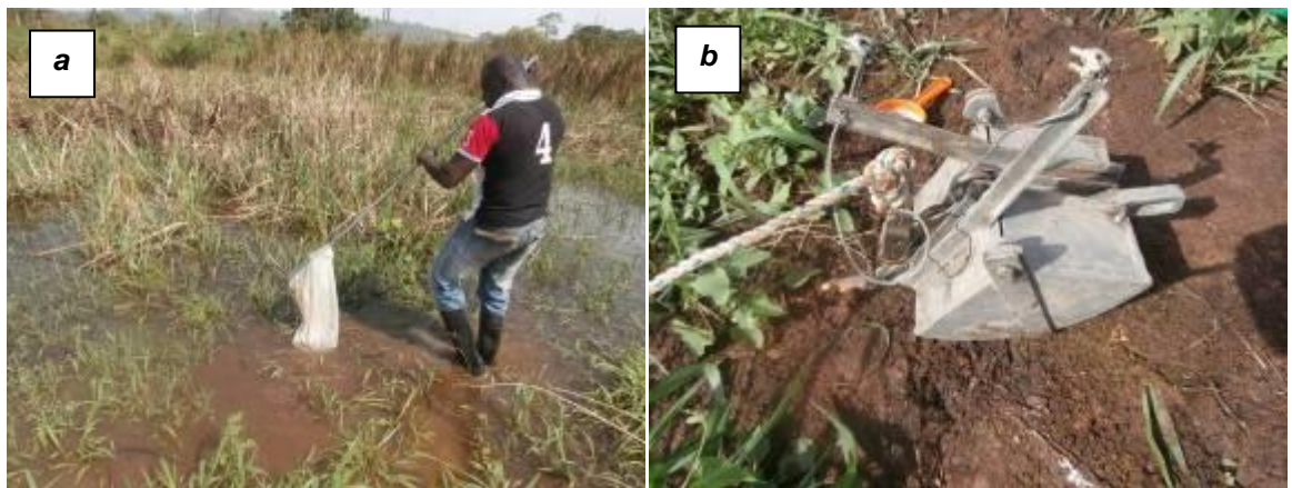
Figure 2-3: Benthic macroinvertebrates sampling: (a) Macroinvertebrate collection session using the kick net; (b) Van Veen grab (Photo: KONAN K. Félix; April 2015)
