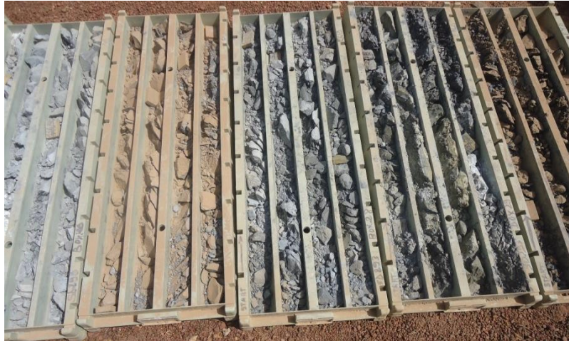
Photo 6 Fracture Zone (aquifer) of 127 m to 153m survey SD293
